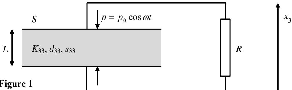
It is convenient to introduce complex variables  $\tilde{p}$ ,  $\tilde{\Delta L}$ , etc., such that:  $p = \text{Re}[\tilde{p}]$ ,  $\Delta L = \text{Re}[\tilde{\Delta L}]$ , etc. In introduced complex variables, the Young modulus is evaluated as:
